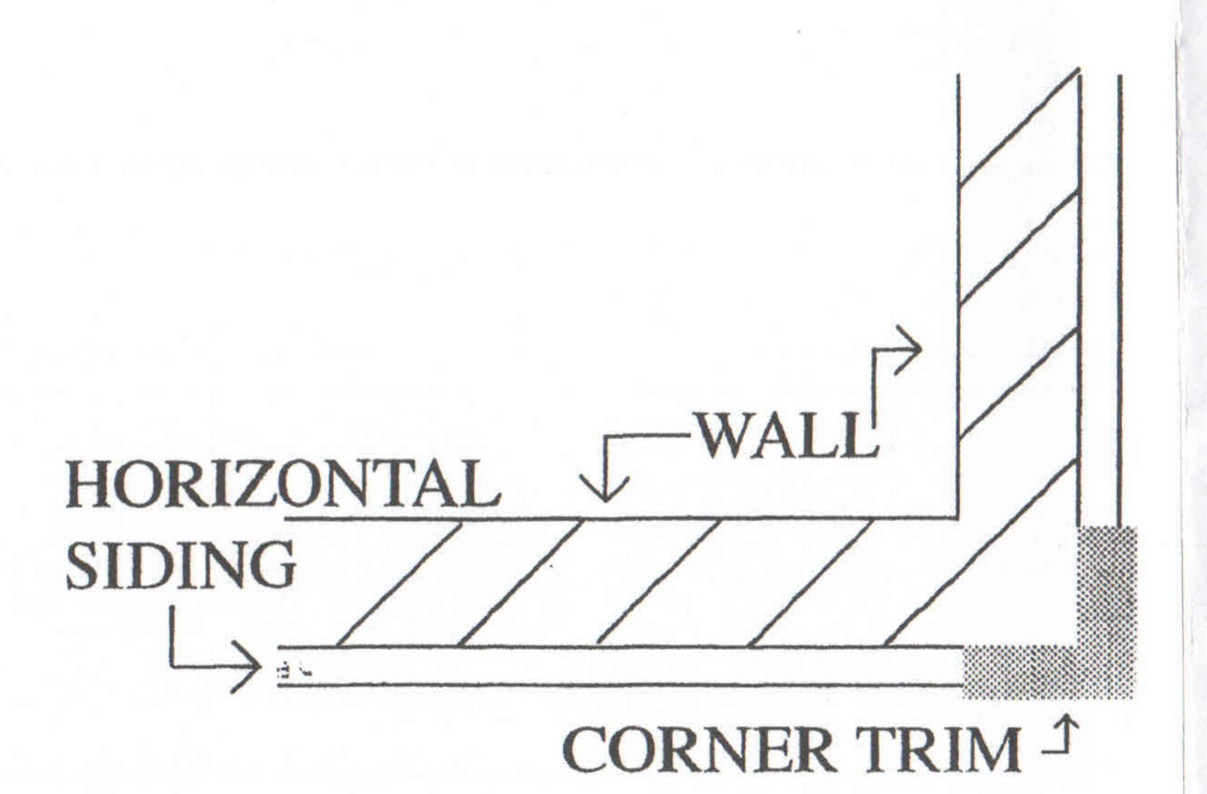
Where horizontal siding is allowed, outside butt miters are prohibited.
